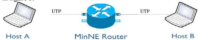
Figure 5. Topology for testing two copper interfaces
