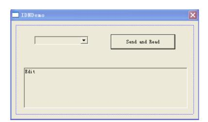
3) Respectively add two variables m\_combox and m\_receive for the controls of Combo Box and Edit Box. See the figure below.
