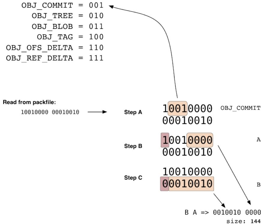
It is important to note that the size specified in the header data is not the size of the data that actually follows, but the size of that data *when expanded*. This is why the offsets in the packfile index are so useful, otherwise you have to expand every object just to tell when the next header starts.
