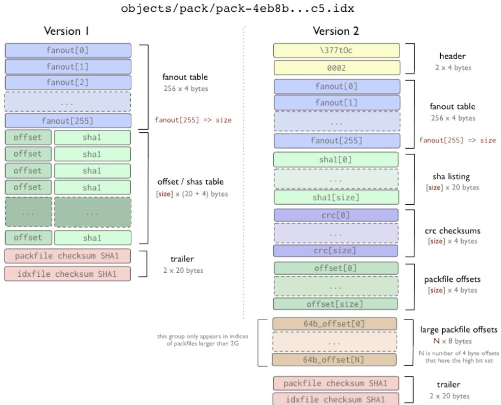
In both formats, the fanout table is simply a way to find the offset of a particular sha faster within the index file. The offset/sha[] tables are sorted by sha[] values (this is to allow binary search of this table), and fanout[] table points at the offset/
