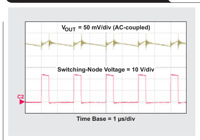
Figure 4. Buck output voltage ripple and switching-node voltage
